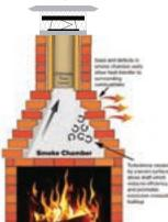
2 The smoke chamber is required to be sealed smooth with refractory mortar to protect exterior combustibles from igniting.
