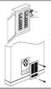
WARNING Take extreme caution when working with electrical heaters. Turn off the electrical power to the heater by switching off the circuit breaker or fuse feeding the heater before removing the grill. Lock, tape or tag the circuit breaker so that the power cannot be turned on accidentally while working on the heater.
