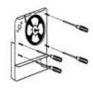
Use a square drive or phillips to remove the four screws that hold the interior cover. Once removed, you have access to the heating element.
