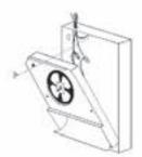
Remove the heater interior from the wall can. To do this: Unfasten the screw at the top of the wall can as shown. 2) Tip the interior forward to expose the power supply connection wires. 3) Disconnect the power wires, making sure you mark them so you can reconnect them exactly the same way, if wires become crossed they could short causing damage. The interior should pull out easily after the mounting screw and electrical connections are removed.
