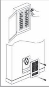
WARNING Take extreme caution when working with electrical heaters. Turn off the electrical power to the heater by switching off the circuit breaker or fuse feeding the heater before removing the grill. Lock, tape or tag the circuit breaker so that the power cannot be turned on accidentally while working on the
