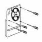
Use a square drive or phillips to remove the four screws that hold the interior cover. Once removed, you have access to the heating element.
