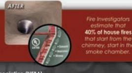
National Fire Protection Association (NFPA) 211 Standard For Chimneys, Fireplaces, Vents, and Solid Fuel Burning Appliances 2010 Edition inner surfaces of the smoke chamber shall be parge coated smooth, with an insulating
